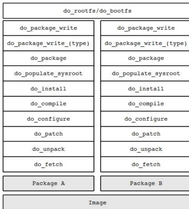
Figure 23.1: High-level overview of Poky task execution
