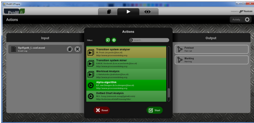
Fig. 10.4 Screenshot of ProM 6. After loading the event log described in Table 7.1, a list of applicable plug-ins is shown and the plug-in implementing the \alpha -algorithm is selected
